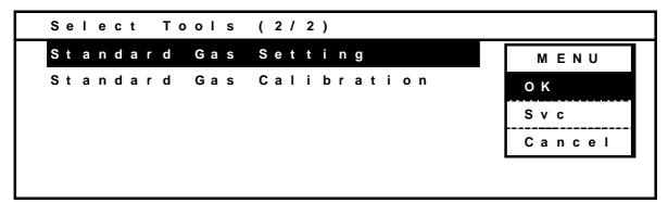
3. Input the  $CO_2$  and  $O_2$  density of standard gas to be used, press the MENU Key to display the menu, select OK, and press the ENTER Key.
